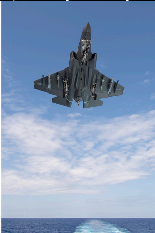
F-35C displaying its hardpoints while taking off from USS Georges Washington ( August 2016)
